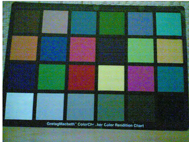
Figure 4 Noisy image taken in +70 degrees Celsius
