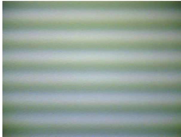
Figure 6 Flicker in an image; object illuminated by strong fluorescent light
